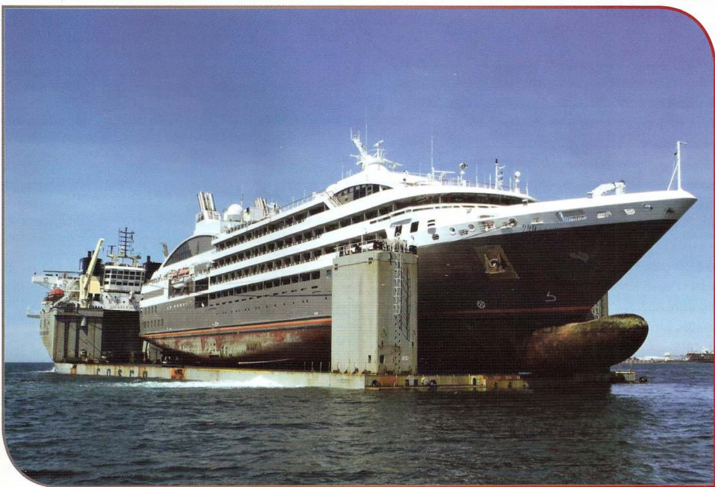
Le Boréal chargé sur HLV Kang Sheng Kou à Punta Arenas, Chili (photo Dutch Offshore Contractors)
