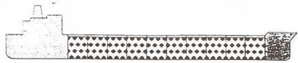
2 After discharging its cargo, quantities of oil remain clinging to the sides of tanks.
