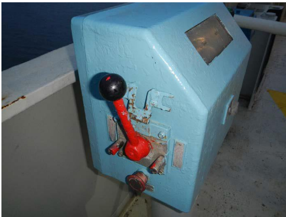
Photo 2: The picture shows the maneuvering lever. By putting a loose piece of equipment it was forced locked into high-speed position. Photo: SHK.
